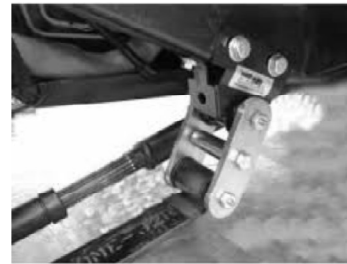
Shackle reversed jeep with arched springs
